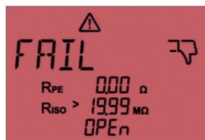
Fig. 47: Failed measurement. "OPEn" is shown on the display. Conductor connection interrupted/switch open
