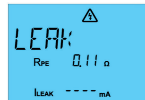
Fig. 59: Protective conductor current measurement in a 3-phase device
