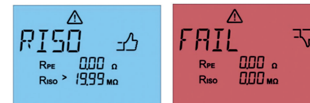
Fig. 44: Passed measurement of insulation resistance (left) and failed measurement (right)
