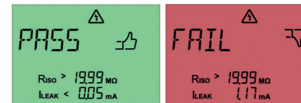
Fig. 33: Passed (left) and failed touch current measurement (right)
