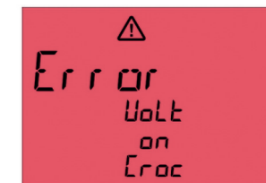
Fig. 61: Voltage on metal parts of the test object
