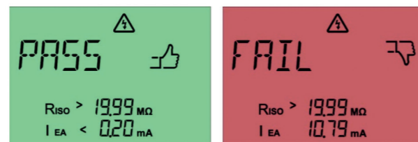
Fig. 35: Passed touch current measurement (left) and failed touch current measurement (right) with the alternative leakage current method
