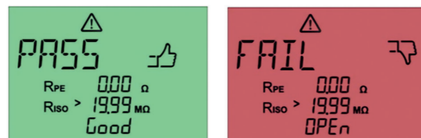
Fig. 49: Final result of a passed line test (left) and a failed line test (right)
