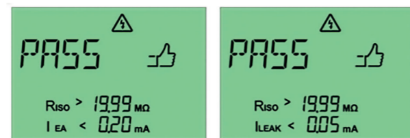
Fig. 36: Passed measurement with the alternative leakage current method (left) and the differential current method (right) for a device with protection rating II
