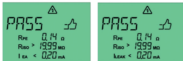
Fig. 26: Passed measurement with the alternative leakage current method (left) and the differential current method (right) for a device with protection rating I
